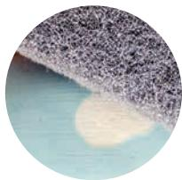
The blue ceramic outer layer contains antimicrobial properties which help the filtration process.
